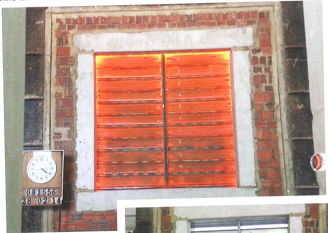
TOP View of the unexposed side of wall mounted damper 4 hours and 20 minutes into the fire test.
