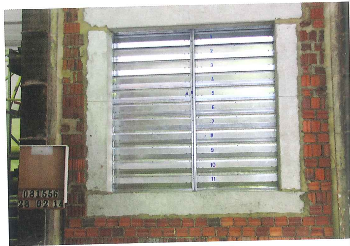
RIGHT, BOTTOM View of the unexposed side of wall mounted damper before testing.
