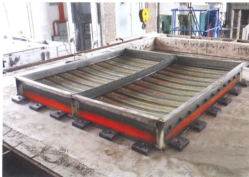
RIGHT BOTTOM View of the unexposed side of a larger single module damper with intermediate frame, damper is floor mounted and is 4 hours and 10 min into the fire test.
