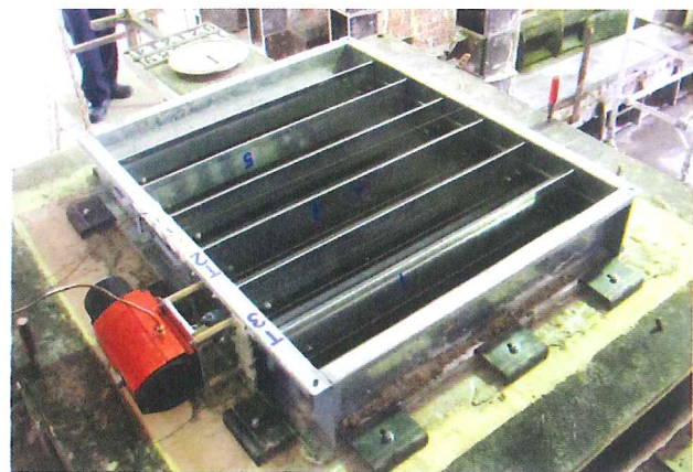
RIGHT, BELOW View of unexposed smaller single module floor mounted damper before testing.
