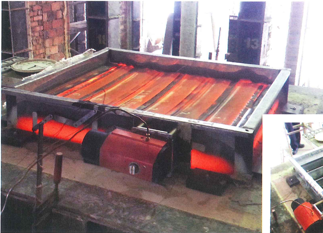
LEFT, TOP Smaller single module floor mounted damper undergoing fire test to BS476 Part 20 and 22.
