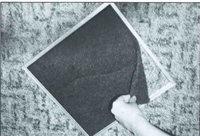
Step 5. Remove the filter media for washing. Note: After washing replace filter in reverse order.
