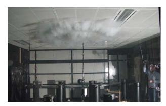
Figure 2: Air flow pattern made visible by smoke tracer
