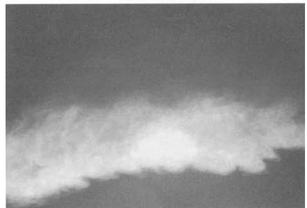
Fig. 7: Low-turbulence horizontal jet spread made visible by smoke tracer; the photographs show the air flow at various points in time after discharge
