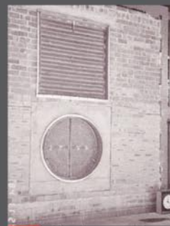
FIG 4D Fire dampers 240 minutes after the start of fire resistance test.
